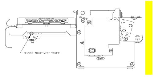
Example adjustment of the moveable side sensor, ITX+ and ITL+.
