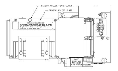
12.4.1.3 Sensor Cleaning Access - ITX 2004AS/3004AS – Adjustable Width Models
