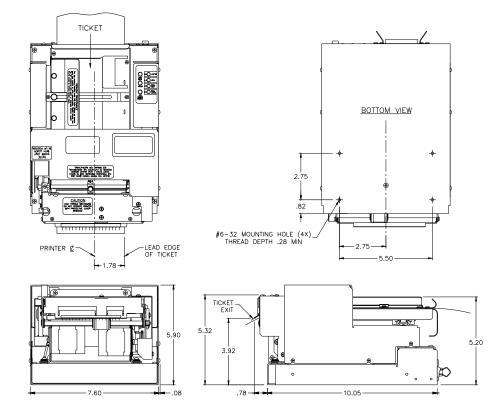
19.2.10 Mechanical Detail Drawing: eITX Desktop Printer (with ticket enclosure cabinet)
