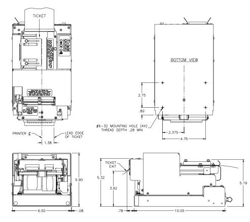
19.2.8 Mechanical Detail Drawing: kITX Kiosk Printer (4.00 – AC Model)
