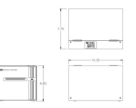
ITX 3000/2000 Printer User Manual (*UMITX315.PDF*) 19.2.3 <u>Mechanical Detail Drawing: pITX Countertop Printer (2.00" and 3.25")</u>
