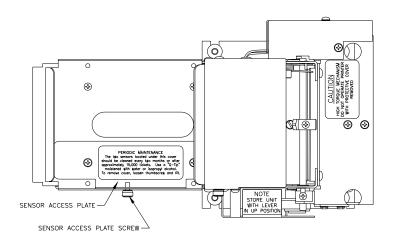
12.4.1.2 Sensor Cleaning Access – ITX 2003A/3003A/2004A/3004A – Adjustable Width Models
