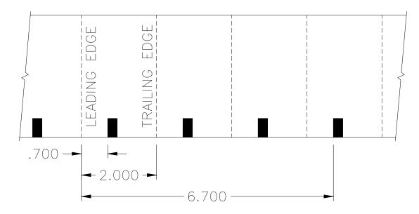
9.1.14 Example 5.5" Length Ticket Drawing for Fixed Width and "AS" Adjustable Width printers
