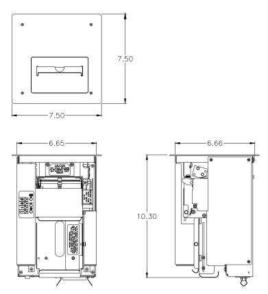
19.2.4 Mechanical Detail Drawing: pITX Countertop Printer (4.00" - AT Model)
